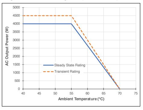
Figure 3: Output Power vs. Ambient Temperature
